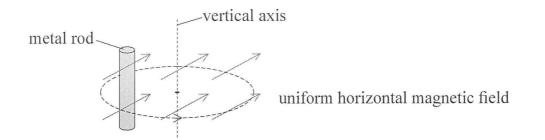
The metal rod completes one circle of radius 0.066 m in 0.020 seconds in the magnetic field of strength 61 mT
