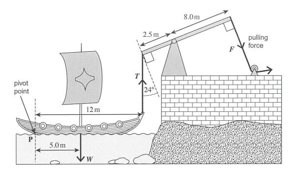
a) Calculate the minimum vertical force **T**, required to start to raise the front of the ship. Assume that the ship pivots about point **P**
