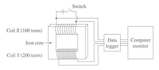
A student closes the switch for a short time, then opens it. The data logger records values of voltage for both coils for the duration of the investigation. The data logger software displays the results as a pair of voltage – time graphs on a computer monitor.
