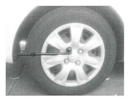
Assuming that it also takes  $3.00 \times 10^2$  Nm to undo the nut, show (by calculation) that if a person of mass 90.0 kg stands on the end of the lever without bouncing, the weight of the person is **not** enough to turn the wheel nut.
