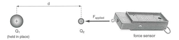
The distance between the charges and the readings on the force sensor are recorded for several different positions. In order to produce a linear plot of the data, the original measurements are adjusted as shown in the table below.
