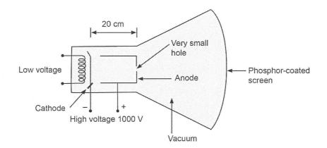
a) Calculate the magnitude and direction of the electric field between the cathode and anode.
