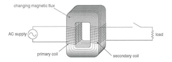
e) One of the major reasons for transformers to have an efficiency less than 100 % is the formation of Eddy currents within the soft iron core of the transformer.
