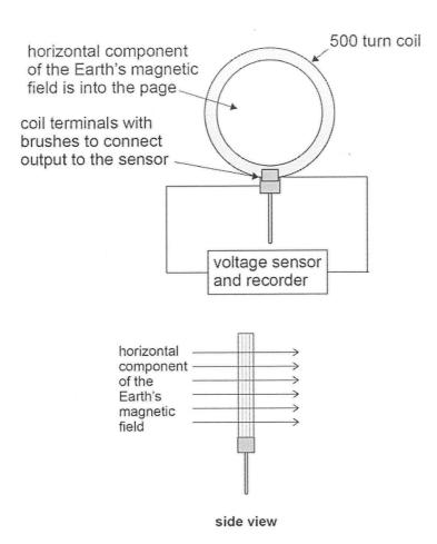
The mean radius of the turns on the coil is 35 cm. The graph below shows how the voltage generated in the coil (V) varies with time when the coil is rotated at 1.5 revolutions per second.
