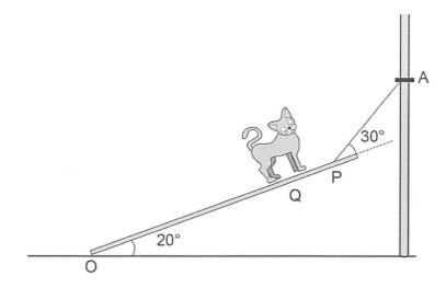
c) Assuming that Point O is the pivot, calculate the tension force in the cable. Show **all** workings.
