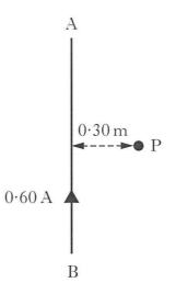
a) Calculate the strength of the magnetic field at point P, a distance of 0.30 m from the conductor. Include an estimate in the **relative error** for the value the magnetic field strength.
